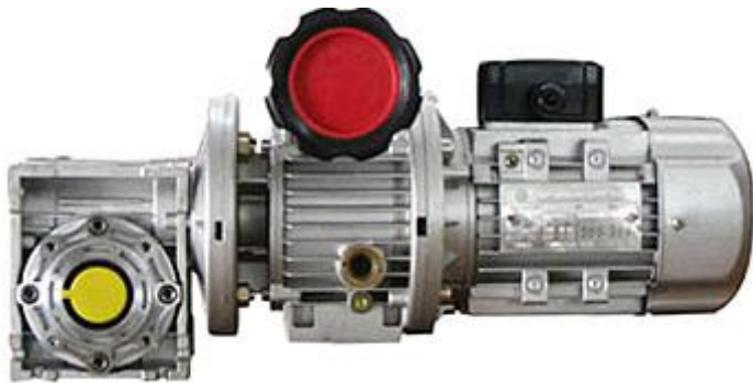
Combination of step less speed reducer and worm gear reducer
